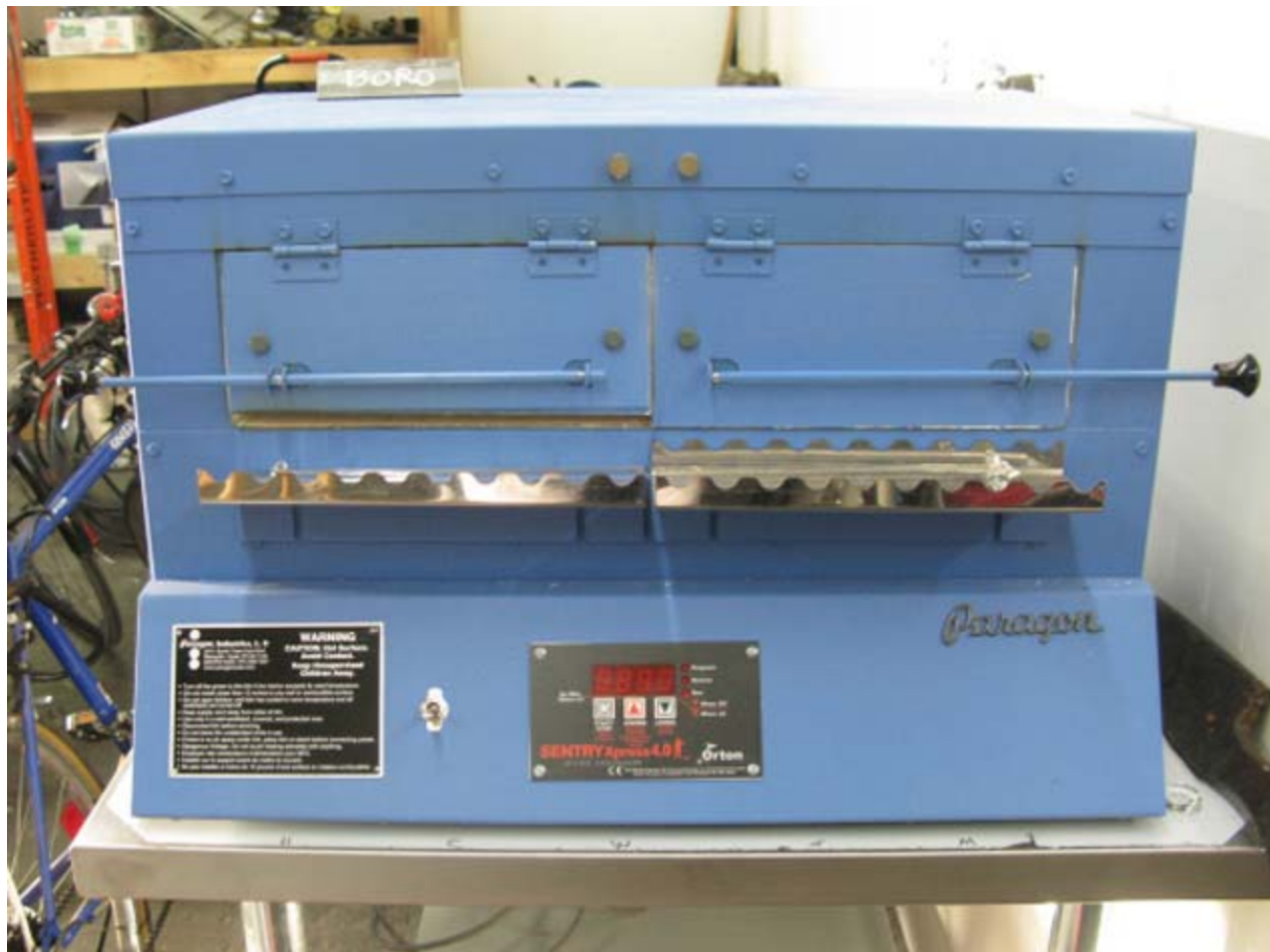
Title: Boro Annealer Photo credit: Larissa Blokhuis Caption: Annealer for flameworking classes.
